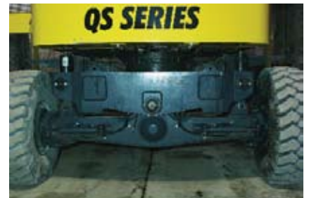
Parker's gas struts help keep the axles on the ground.
